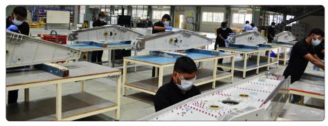
Airbus A330 Flap Track Beam Assembly Line at Dynamatic Aerotropolis
