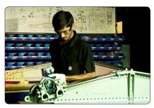
Assembly of Flap-Track-Beams for Airbus A320 Single Aisle Aircraft at Dynamatic, Bangalore, India
