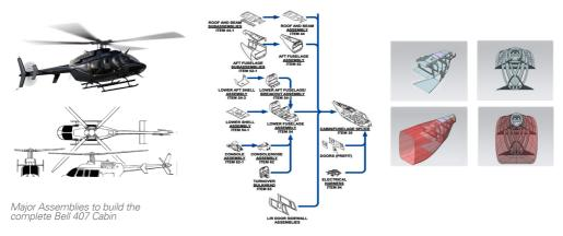
The industrialisation program at Dynamatic has involved digitisation of over 2000 detail parts, followed by development of tooling, processes and part manufacturing. We have now taken up the 5 major fuselage assemblies and has supplied over 407 ship sets.
