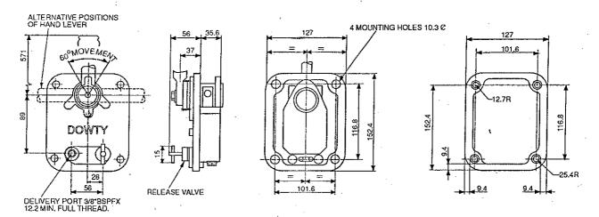
INSTALLATION NOTE: UNITS MUST BE INSTALLED IN THE POSITION SHOWN, THAT IS, IN THE VERTICAL POSITION WITH THE HANDLE PIVOT ABOVE THE DELIVERY PORT.
